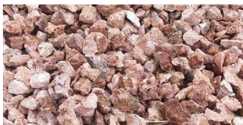
Figure 1. Substandard limestone aggregate from Meleura Village, Muna Regency, Southeast Sulawesi
